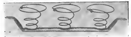
CARDINAL METHOD OF SPRING ASSEMBLY.
